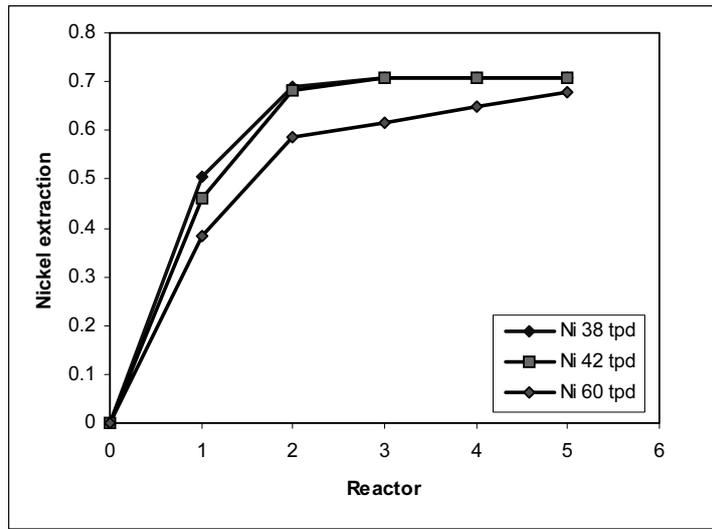
Figure 3. Nickel extraction as a function of capacity.
