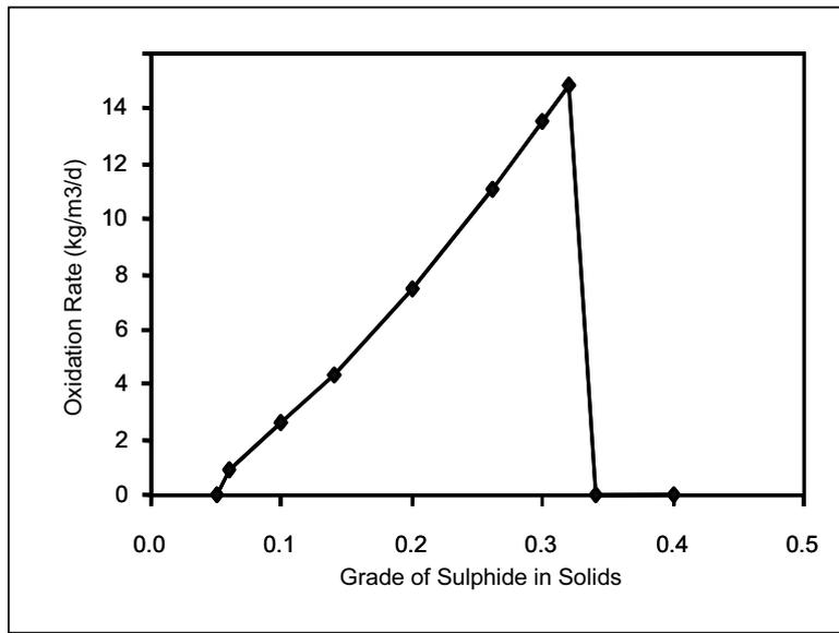
Figure 9: The effect of increasing the sulphide load on the performance of a leaching reactor.
