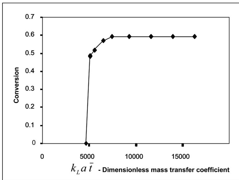
Figure 8: The effect of the mass transfer coefficient on the performance of a leaching reactor.
