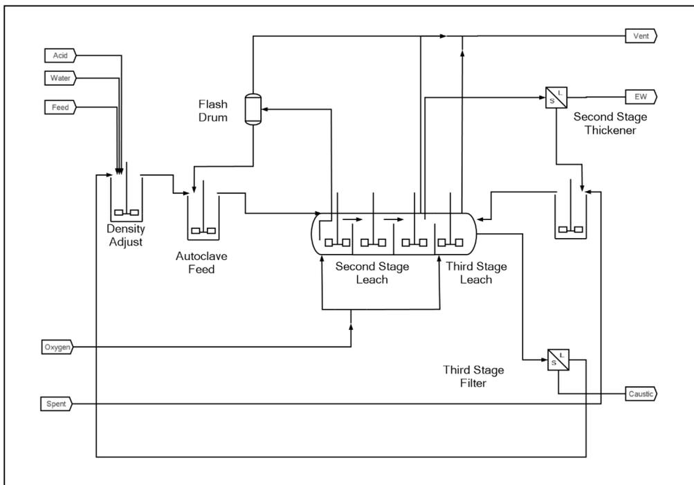
Figure 5: Second and third stage autoclave configuration.
