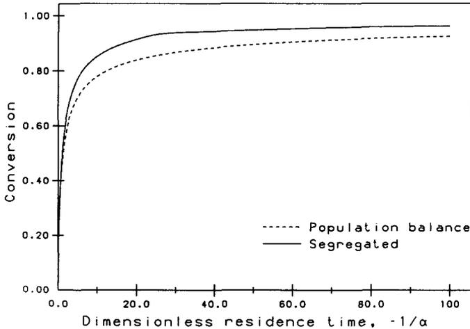
Fig. 1. The conversion calculated from the segregated-flow model (Eq. 5 and 6) and the population-balance model (Eqs. 7–11) for a single ideally-mixed tank. The amount of leaching reactant,  $B$ , is in stoichiometric proportion to the amount of mineral in the feed. The reaction kinetics are described by Eq. (13).
