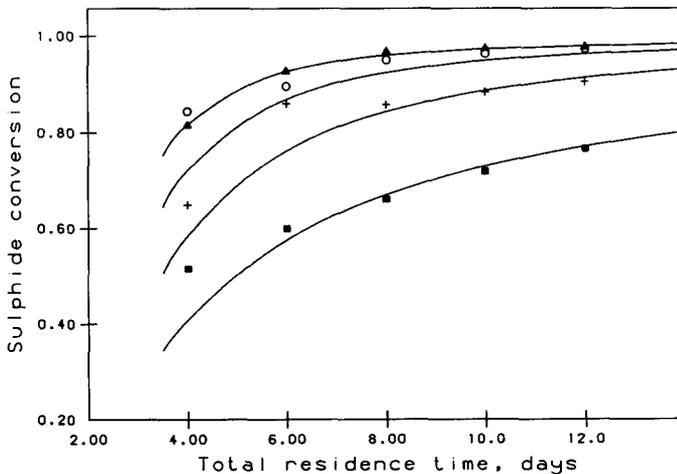
Fig. 3. The bacterial leaching of a gold-bearing pyrite concentrate in a series of continuous reactors. The data are from Miller [28,29] and the lines represent the model, given by Eqs. (7), (24) and (25). The parameters for the model were those determined from the batch experiments and are given in Table 2.
