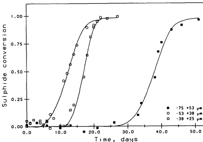
Fig. 2. The bacterial leaching of a gold-bearing pyrite concentrate in a batch reactor. The data are from Miller [28,29] and the lines represent the solution to the model, given by Eq. (23). The parameters for Eq. (23) are given in Table 2.
