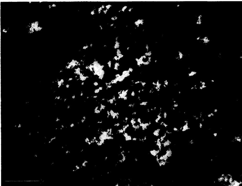
Fig.5 The fluorescent image of the biofilm, indicating the non-uniform coverage of the surface after two days for the same area shown in Figure 4. The length of the scale bar is 100  $\mu\text{m}$
