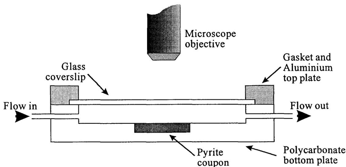
Fig.2 Diagram of the flow cell
